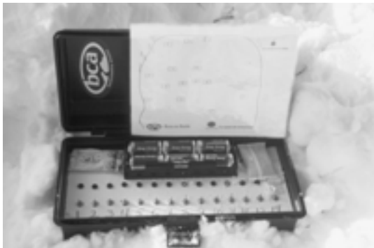
Beacon Basin control panel.
