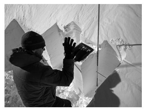
Figure 10: Compression test technique and column dimensions.
