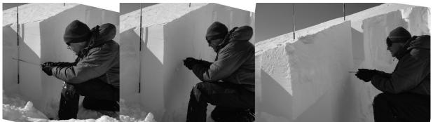
**Figure 13b:** Another PST example with result recorded as "PST 45/100 (End) down 42cm on SH 4.0 100724".
